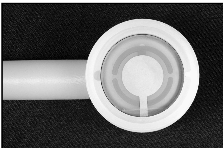
Figure 9. Crystal in place with correct electrode orientation.
